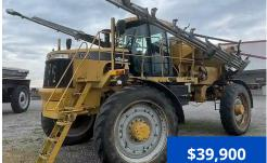
2011 Ag Chem Rogator 1396, 4905 hrs., Caterpillar 365 hp diesel engine, hydrostatic trans., painted 409SS AGCO Airmaxx spreader 200 ft3, 60 ft booms, A/C, AM/FM radio, 380/90R46 tires (30% remains), includes a set of floater tires.
