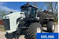
2013 GVM E325 Prowler, 3850 hours, Cummins QSL 8.9 hp turbo diesel engine, ZF 6-speed trans., 304 SS New Leader spreader, Raven Viper Pro, A/C, AM/FM radio, air ride seat, front 650/65R32 rear 800/65R32 BKT tires (90% remains).
