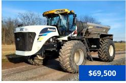
2011 GVM E350 Prowler, 2192 hrs., mechanically friendly, Cummins 8.9L 350 hp diesel engine, automatic Funk DF250 trans., 11-ton 304 SS GVM Double Duty Fusion Ready body with 5 ft. Fusion insert, Raven Viper Pro, AutoSteer, RGL 600 lightbar, AM/FM, A/C, air ride seat, 380/105R50 row crops not pictured.
