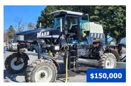
**2016 GVM Mako 400HC**, 681 hrs., Cummins Tier III QSB4.5L 130 hp diesel engine, Allison auto. 2100 RDS trans., 46 in. clearance, double telescoping drive shaft, 400 gal. poly tank, 80 ft booms, 5-section shutoff valve, rotary triple nozzles, 20 in. nozzle spacing, Ag Leader Incommand 1200 with 7500 GPS, Ag Leader SteerCommand, RTK unlocked, Greentronics, air ride seat, A/C and heat, AM/FM/BT radio, toolbox, front and rear fenders, 380/85R24 tires.
