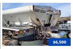
**2013 New Leader L3220G4**, painted 409 SS New Leader L3220G4 12 ft. spreader body, 250 cu ft capacity, fenders, 34 in belt over chain, multiplier ready, Raven product control node. No hydraulic tank and cooler.
