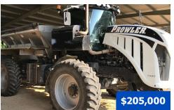
**2019 GVM T380 Prowler,** 1882 hrs., Cummins QSL9 380 hp turbo diesel engine, Funk DF250 4x4 powershift 11-speed auto. trans., 114 in. Dromos axles rated @ 32,000 lb., 4WS, reverse pitch fan, 304SS 9.0T New Leader NL5000G5 spreader body, Raven Viper 4 with RS-1 ISO steering receiver, A/C, AM/FM/BT radio, air ride seat, window tint, roll tarp, front fenders, 380/90R46 Trelleborg tires (90% remains). EPG warranty options available. SN: CS-193804WT1029 (MO) **U1556**
