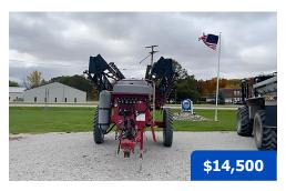
**2010 Redball 670,** 1200 gal. poly tank, 90/60 ft booms, 5-section shutoff valve, rotary triple nozzles, 20 in. nozzle spacing, Raven SCS 460 controller, Ace hydraulic pump, catwalk, 320/90R46 tires (80% remains).
