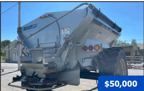
**2015 GVM 8.0T Double Duty FR Pull Spreader**, 409 SS GVM Double Duty 8.0-ton 10 ft. spreader body, fusion ready, Raven ISOBus compatible with any VT terminal, 10 ft x 102 in. wide, 250 ft<sup>3</sup> capacity, Cable-Lok roll tarp, 120 in. track frame assembly, (2) 380/95R46 Trelleborg tires (70% remains), includes Scale-Tec (4) load cell system with monitor.
