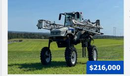
**2022 GVM Mako 455,** 290 hrs., Cummins Stage V 3.8L 130 hp diesel engine, Allison auto. 2100 RDS trans., 46 in. clearance, double telescoping drive shaft, 425 gal. poly tank, 42/80 ft Pommier booms, 5-section shutoff valve, rotary triple nozzles, 15 in. nozzle spacing, Patchworks, Greentronics, EVO spray safe cab, air ride seat, A/C and heat, AM/FM/BT radio, LED work lights, rotating beacon, 320/85R24 front 380/85R24 rear tires.
