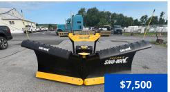
**2023 Sno Way 29HD V-Plow,** 8 ft. adjustable steel blade, down pressure series 2-29HD power pack, LED thermosensitive heated lights, wireless controller for plow and lights, upgraded hydraulics package, outboard mount stand, complete fleet 2-plug connection system, energy smart system, set of plow shoes, includes emergency parts repair kit.
