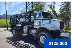
2016 Peterbilt Stahly PB348, 1320 hours, 11,429 miles, Peteriblt chassis, PX-9 350 hp diesel engine, automatic trans., 1450 gal. SS tank, 80 ft booms with SS boom lines, 20 in. nozzle spacing, 5-section shutoff valve, 5-body nozzles, Rayen Viper 4 controller, foam marker, AM/FM, A/C, air ride seat, fenders, front 48x25.00-20 Michelin (80% remains) rear 66x43.00-25 Alliance tires (70% remains). Includes set of row crop tires (90% remains). Excellent Condition!
