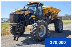
2014 Rogator RG1300, 2793 hours, AGCO 8.4L 330 hp turbo diesel engine, 4WS, painted 409 SS New Leader L4258G4, Raven Viper Pro, Phoenix 300 GPS, parallel swathing, air ride seat, A/C, beacon lights, fenders, electric roll tarp, Michelin 380/90R46 tires (front 45%, rear 35% remains), Goodyear 650/65R38 (30% remains).
