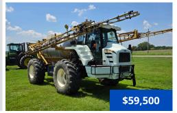
2012 GVM 9275 Prowler, 5921 hours, Cummins QSB6.7L 275 hp diesel engine, Funk 10-speed powershift trans., 114 in Axletech axles, 1600 gal. SS tank, 70/90 ft booms with SS boom lines, 15 in. nozzle spacing, 5-section shutoff valve, triple body nozzles, Raven Envisio Pro, Accuboom, A/C, AM/FM radio, air ride seat, 380/90R46 row crop tires (30% remains). Floaters not included.
