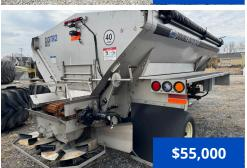
2025 GVM Double Duty TR2, 11 ton, 13 ft x 102 in., 330 cu. ft. capacity, designed for lime and fertilizer spreading, 304 SS cross member and mount, peaked end plates, PWM valves with RCM ISO spinner and drag controls, Reverse Rotation spinners, twin 16 in. #3 conveyor chain with wiper, dual conveyor rate sensors and bulkhead window, 304 SS frame cover, 124 in. float fenders, and rear camera.
