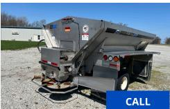
**2021 GVM Double Duty SS1,** 11 ton, 13 ft x 102 in. wide, 330 ft<sup>3</sup> capacity, 304 SS cross member and mounts, peaked end plates, PWM valves with RCM ISO spinner and drag controls, Heavy Bulk Standard Rotation spinners, 34 in. #3 conveyor chain with wiper, rate sensor, bulkhead window, 304 SS frame cover, 124 in. float fenders, and rear camera.
