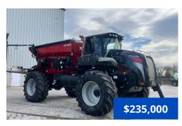
2022 RBR Vector 430, 901 hrs., Cummins 430 hp 9L diesel engine, Allison Automatic transmission, Marmon-Harrington 4x4 drop box, Raven Viper 4+, RS1 antenna, Raven Autosteer, 710/70R38 Floater tires (75% remains), 380/90R46 Row Crop Tires (50% remains). Chassis only.
