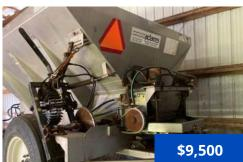
Adams HLS-6-2W. 304 SS pull behind fertilizer spreader, lime and fertilizer, single axle, high ground clearance, hydraulic spinners, row crop spread axle on 30 in. center, twin spinner, ground drive, hydraulic press wheel engagement, nice stainless box, brand new tires.
