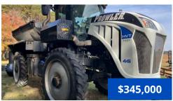
2022 GVM T325 Prowler, 667 hrs., Cummins B6.7L 325 hp turbo diesel engine, Dana HVT-R2 trans., adjustable axles, 4WS, 304SS GVM 11.0T Double Duty TS2 spreader body, 2-section shutoff, bulkhead window, 124 in. fenders, Raven Viper 4+ with RS-1 ISO steering receiver, RGL 600 light bar, A/C, AM/FM/BT radio, air ride seat, window tint, roll tarp, 380/90R46 row crop tires (60% remains). Includes remainder of 3-yr/3000 hrs. EPG Premier Warranty.
